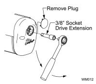
3. Turn the handle counterclockwise until the awning is retracted.
