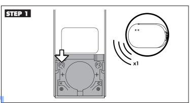
• Press the P2 button on the remote. The receiver beeps once.
