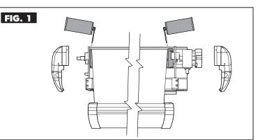
Spray silicone lubricant on the moving parts of the awning.
