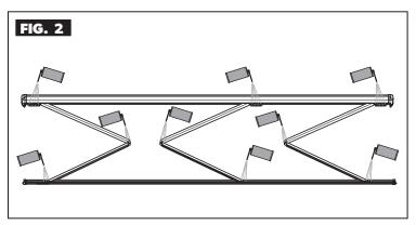
• Spray silicone lubricant at the joints of the arm assemblies.
