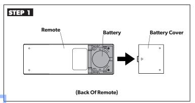
• Insert one CR2430 Li-MnO2 battery. Replace battery cover.
