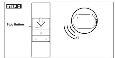
• Press the Stop Button on the remote. The receiver beeps once.
