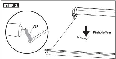
**NOTICE NEVER** close (roll up) awning when vinyl liquid patch (VLP) is wet. Otherwise, damage to other parts of the awning fabric (melting through layers) will occur.
