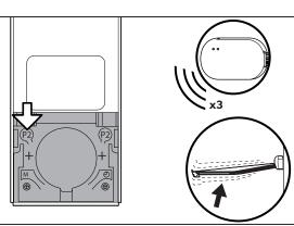
Press the P2 button on the remote. The receiver beeps three times and the awning jogs.
