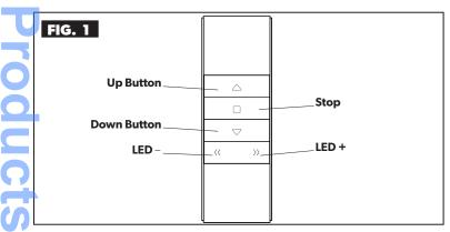
• Press the UP and DOWN awning remote buttons to retract and extend the awning.
