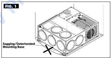
Confirm the Furnace mounting base is not sagging or deteriorating.
